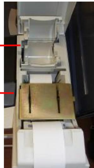
14. Insert the end of the paper into the slot on the Security Canister Spool and wind it as shown on the spool. Return the spool to the Security Canister and close the Security Canister securely.
