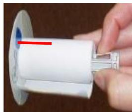
9. Put a new paper roll (provided in your touch screen voting unit supplies) on the paper spool with the spool wheel on the left and the paper coming from the bottom.
